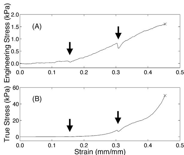
**Figure 9.** Stress-strain relationship of the tissue-derived biomaterial expressed in terms of engineering stress (A) and true stress (B). Arrows denote stress-relaxation response of the specimen due to an interruption in mechanical loading to accommodate image collection.
