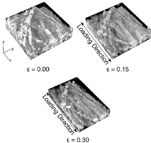
**Figure 7.** Three-dimensional reconstructed confocal reflection images show deformation of microstructure within the tissue-derived biomaterial under unloaded and loaded (applied strain levels of 0.15 mm/mm and 0.30 mm/mm) conditions.
