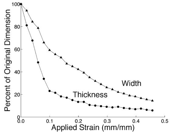
**Figure 5.** Width ( $\blacktriangle$ ) and thickness ( $\bullet$ ) measurements of a reconstituted type I collagen matrix (1.0 mg/ml type I collagen polymerized under physiologic conditions) at various levels of applied strain. Values are expressed as a percentage of original specimen dimensions (no applied strain).
