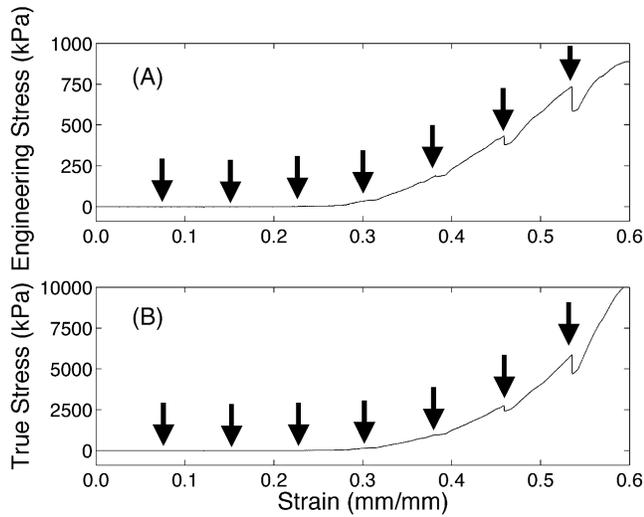
**Figure 6.** Stress–strain relationship of a three-dimensional ECM construct (1.0 mg/ml type I collagen polymerized under physiologic conditions) expressed in terms of engineering stress (A) and true stress (B). Arrows denote stress-relaxation response of the specimen due to an interruption in mechanical loading to accommodate image collection.
